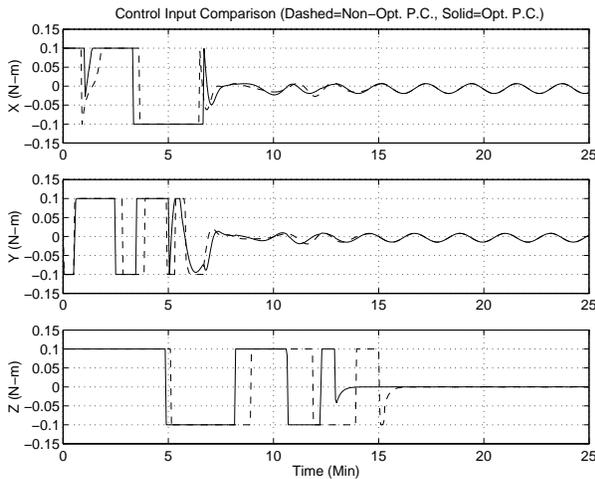
**Fig. 3 Optimal and Non-Optimal Predictive Control**
