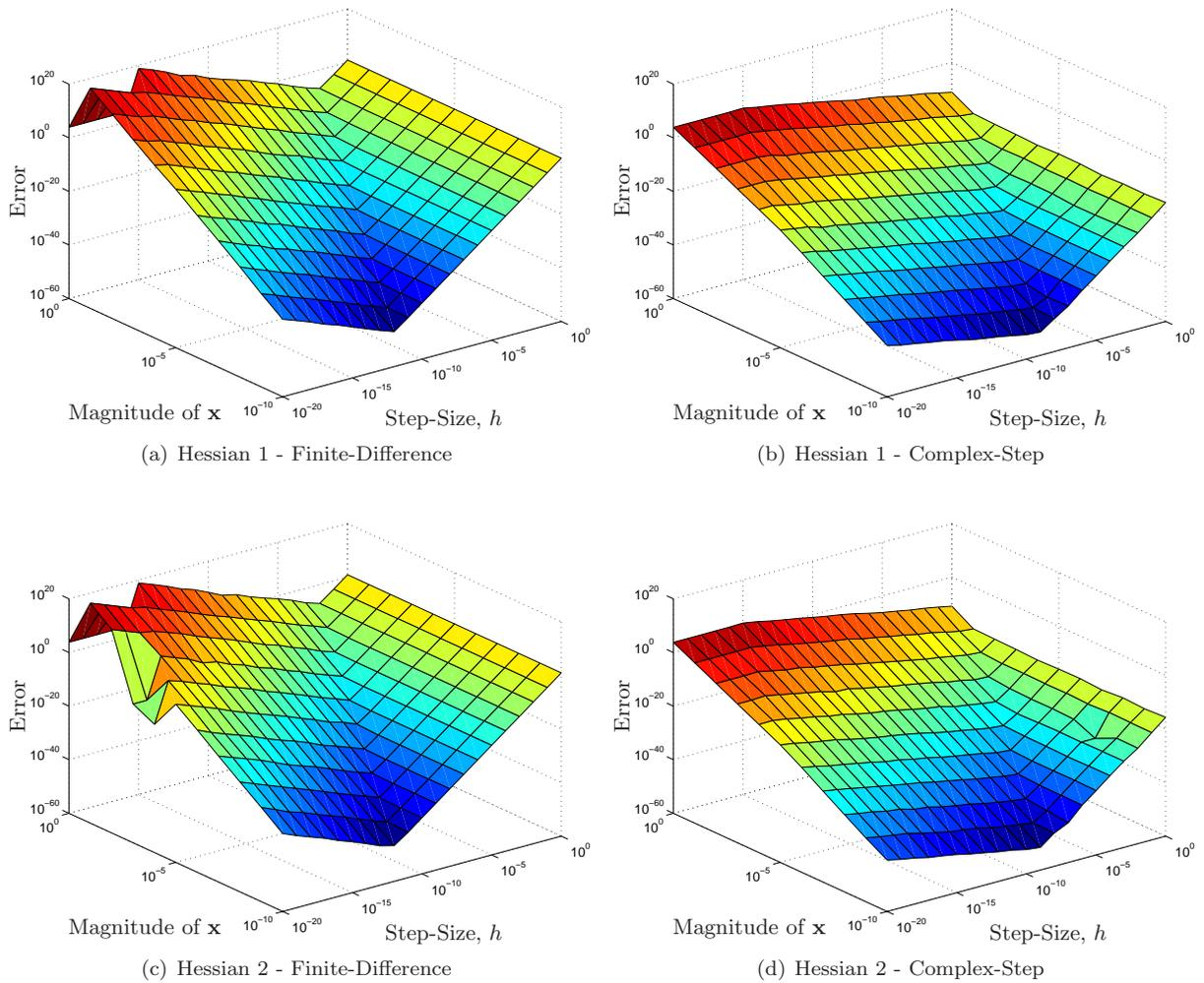
Figure 10. Infinity Norm of the Hessian Error Matrix for Different Magnitudes and Step-Sizes
