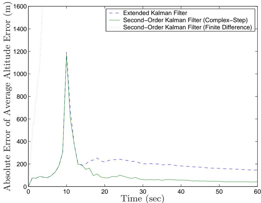
Figure 12. Absolute Mean Position Error
