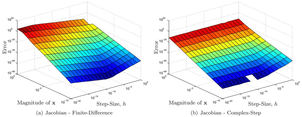
Figure 9. Infinity Norm of the Jacobian Error Matrix for Different Magnitudes and Step-Sizes
