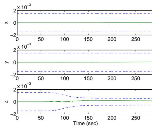
(f) Accelerometer-Scale Factor Errors and  $3\sigma$  Bounds
