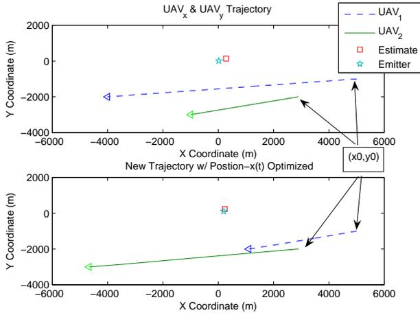
Figure 7: Velocity Control Simulation: UAV Trajectories
