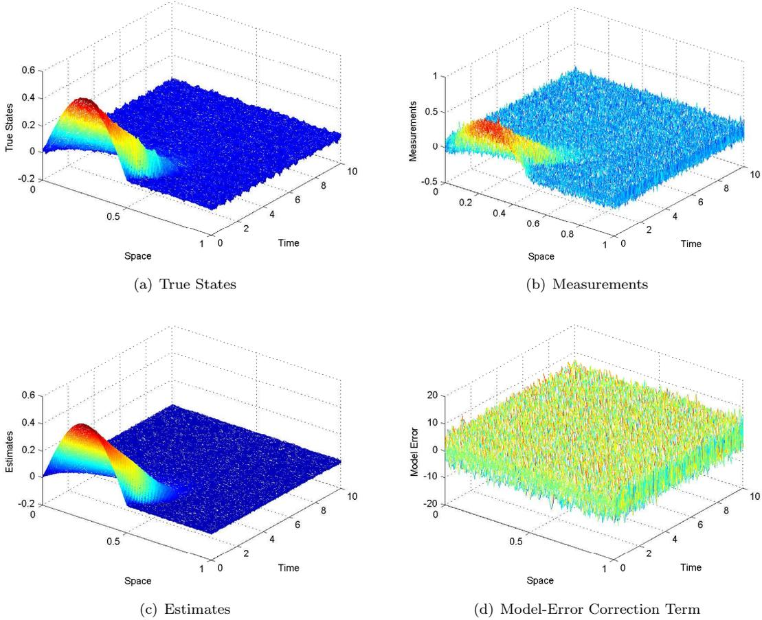
**Figure 7. Full-Order Control; Noise, with Model-Error Correction, Kalman Filter,  $N_m = 101$ ,  $\kappa = 0.001$**
