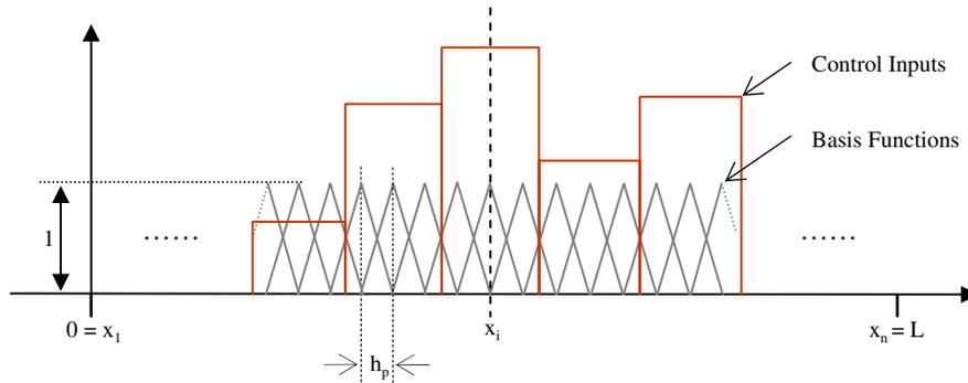
**Figure 3. Distributed Control with High Order Basis Functions**
