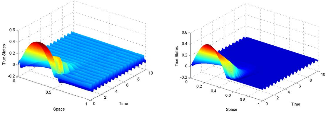
(a) True States; Noise; Kalman Filter; No Model-Error Correction (b) True States; No Noise; Active ‘Filtered’ Model-Error Correction
