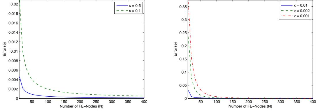
(a) Averaged Error per Gridpoint between FEM and Analytical Solution (b) Averaged Error per Gridpoint between  $w^N$  and  $w^{2N}$
