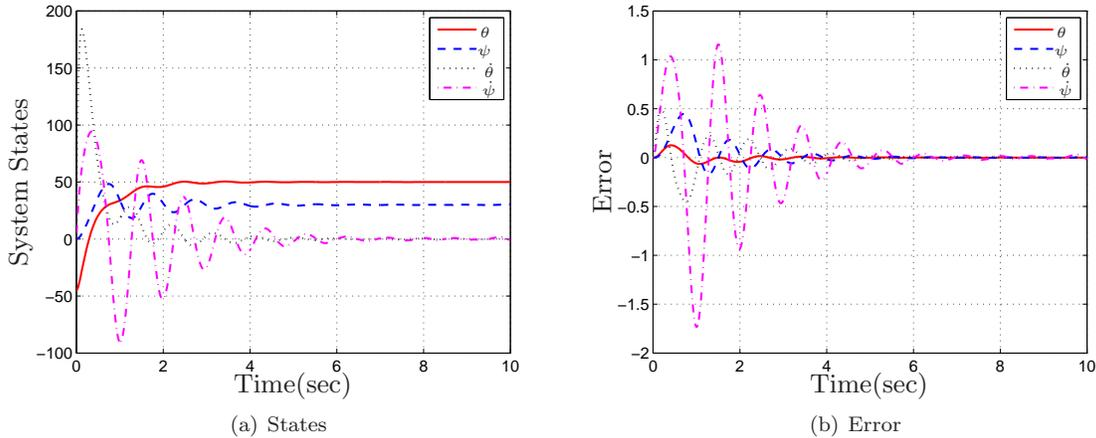
**Figure 2. Unsaturated Adaptive Disturbance Accommodating Control Results: Actual States and Error**
