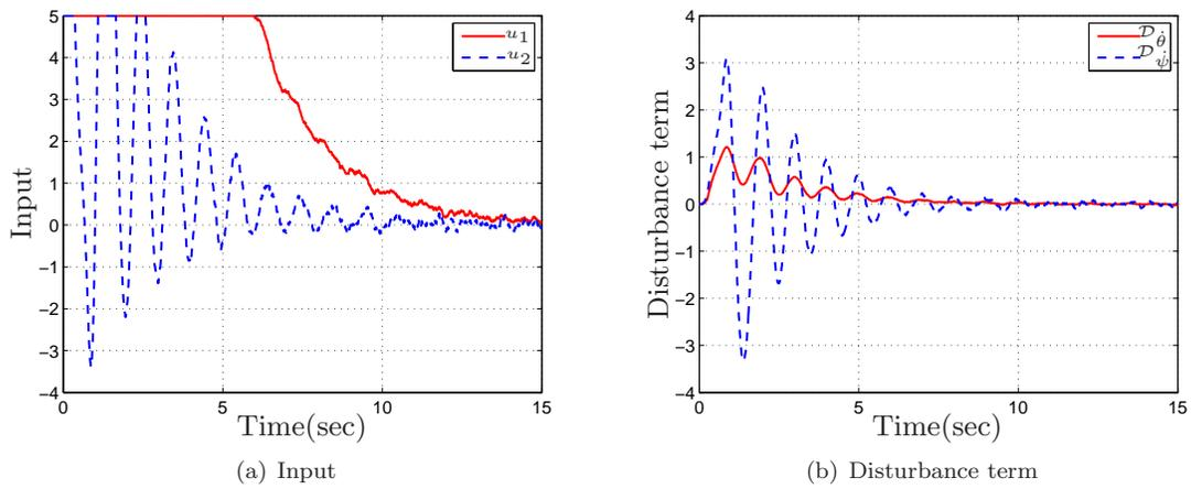
Figure 7. Saturated Adaptive Disturbance Accommodating Control with Adaptive Feedback Gain: Control Input and Estimated Disturbance term
