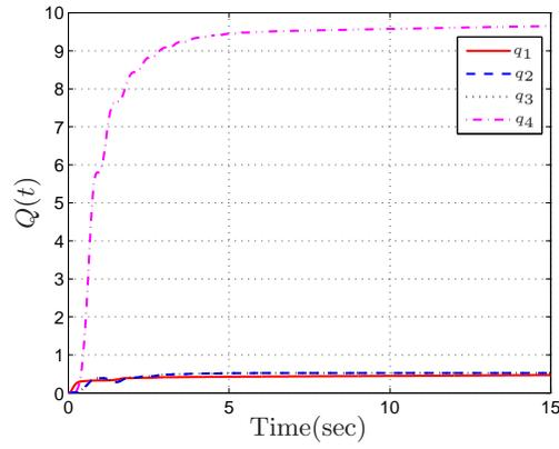
Figure 8. Saturated Adaptive Disturbance Accommodating Control with Adaptive Feedback Gain: Adaptive  $Q(t)$
