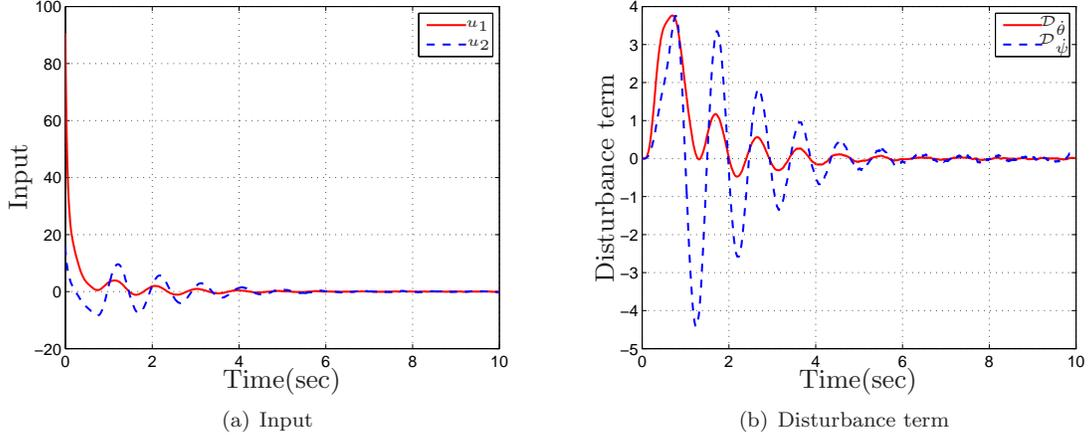
Figure 3. Unsaturated Adaptive Disturbance Accommodating Control Results: Control Input and Estimated Disturbance term
