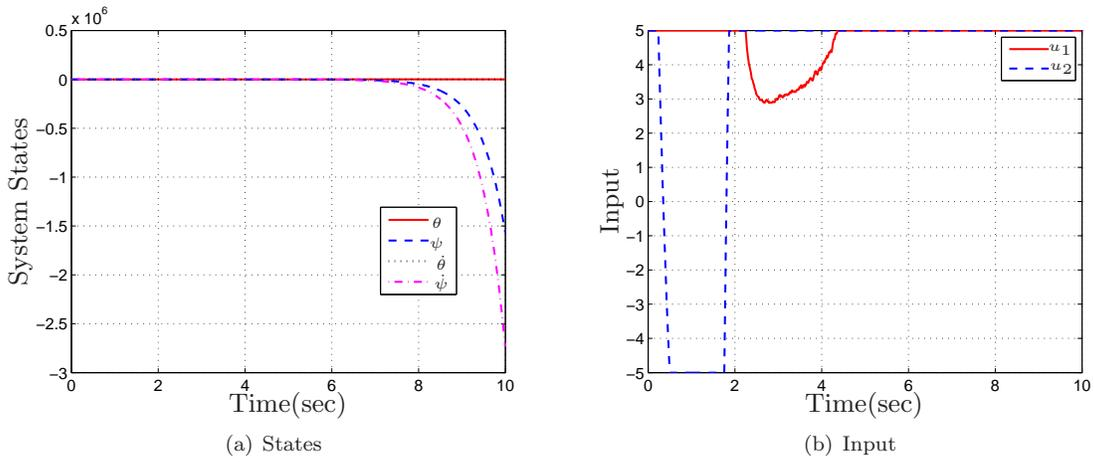
Figure 5. Saturated Adaptive Disturbance Accommodating Control Results: Actual States and Control Input
