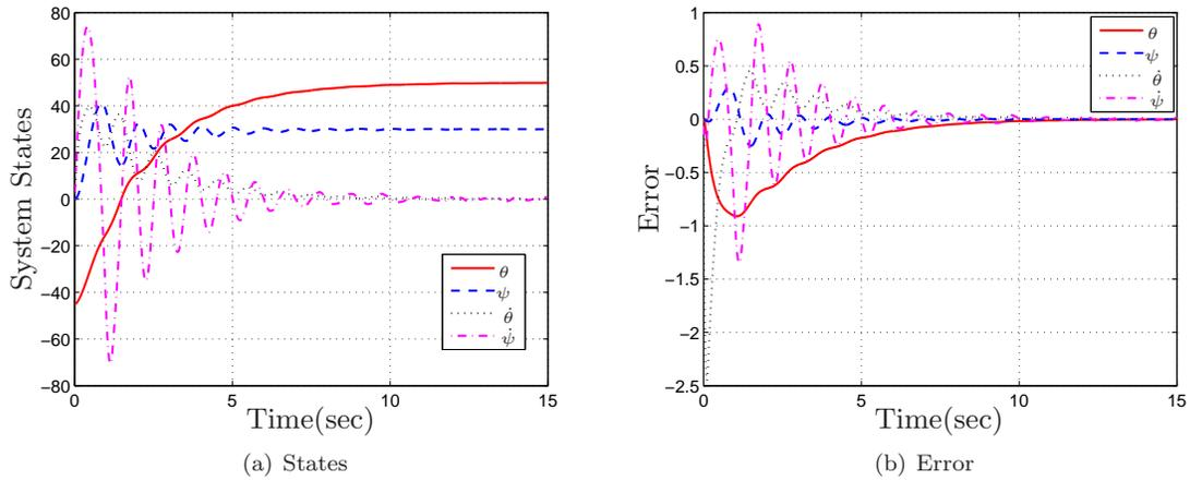
Figure 6. Saturated Adaptive Disturbance Accommodating Control with Adaptive Feedback Gain: Actual States and Error
