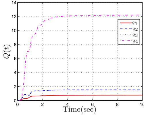
Figure 4. Unsaturated Adaptive Disturbance Accommodating Control Results: Adaptive  $Q(t)$
