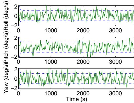
(b) MMAE Angular Rate Errors and  $3\sigma$  Bounds
