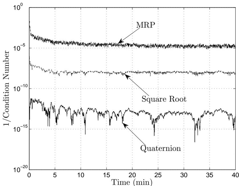
Figure 4. Inverse Condition Number for the Quaternion and Local Error MRP Algorithms
