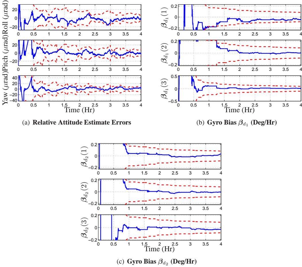
Figure 6. Relative Attitude Estimate Errors for the Filtering Cases
