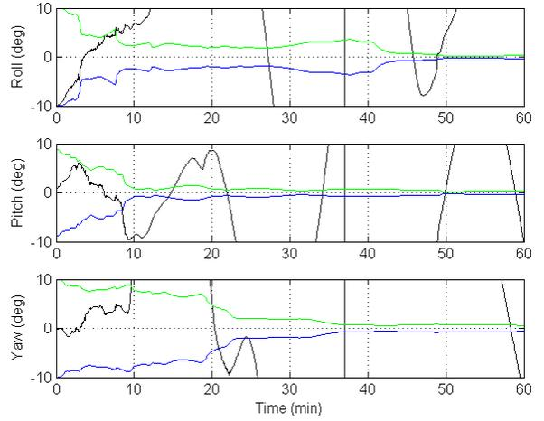
Fig. 11. Attitude difference from truth and 3- $\sigma$  error bounds for Test #3
