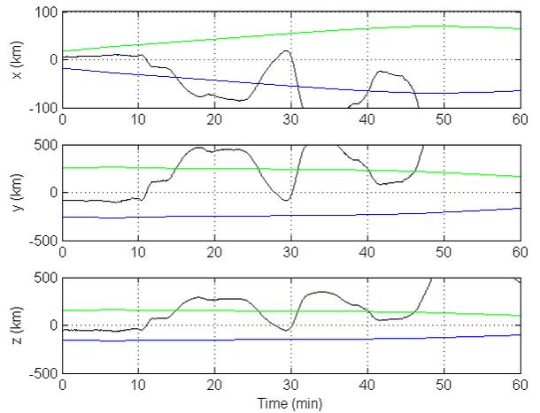
Fig. 13. Position difference from truth and 3- $\sigma$  error bounds for Test #3
