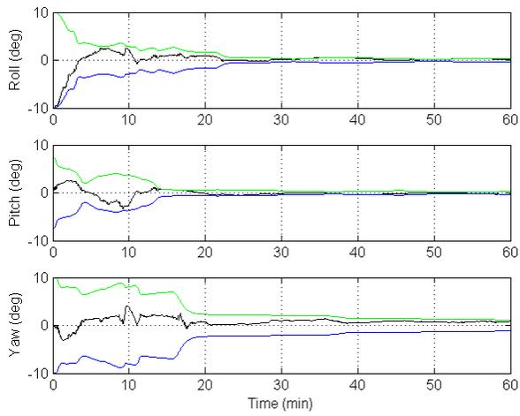
Fig. 5. Attitude difference from truth and 3- $\sigma$  error bounds for Test #1
