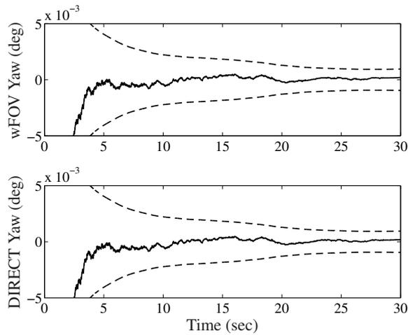
Figure 4. Yaw-Axis Errors with  $3\sigma$  Bounds
