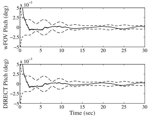
Figure 3. Pitch-Axis Errors with  $3\sigma$  Bounds
