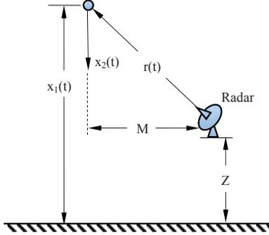
Fig. 1. Geometry of the Vertically Falling Body Example
