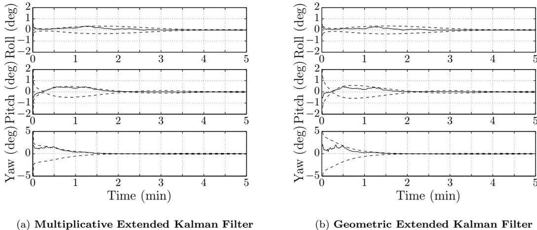
Figure 5. Transient Attitude Errors and 3-Sigma Bounds for the MEKF and GEKF
