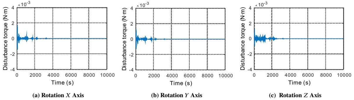
**Fig. 18 Reaction wheel disturbance torques with SMC controller and adaptive moment distribution algorithm.**
