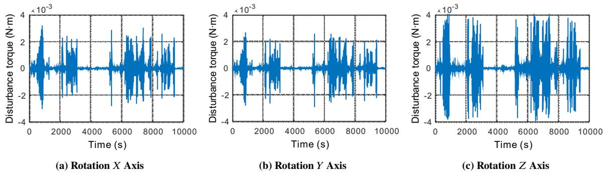
**Fig. 9 Reaction wheel disturbance torques with PD controller.**
