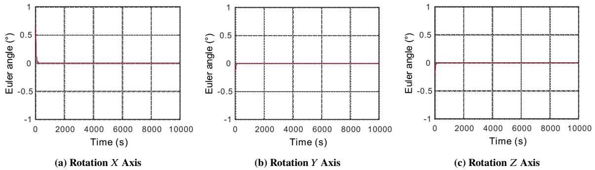
**Fig. 13 Euler angle histories with PD controller and adaptive moment distribution algorithm.**
