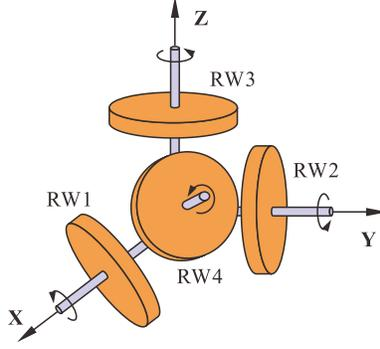
**Fig. 5 Configuration of the RWA.**
