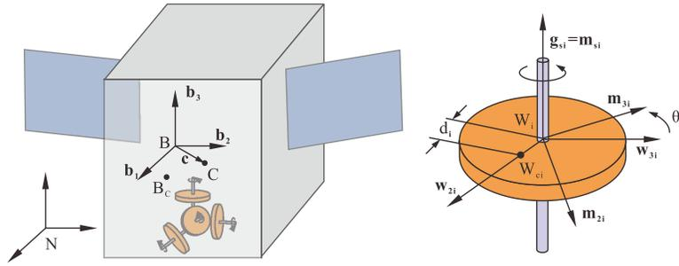
**Fig. 4 Variables and reference frame definitions.**
