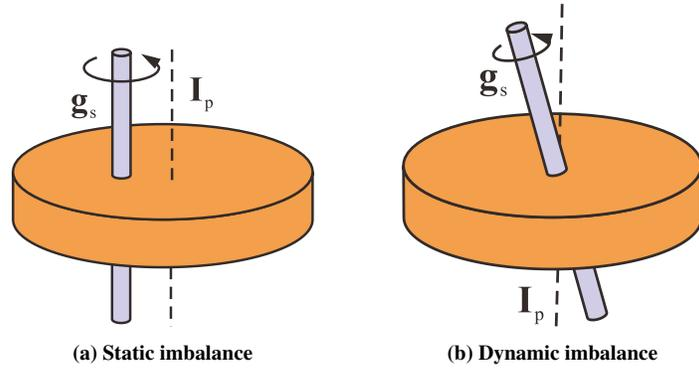
**Fig. 3 Imbalance of a reaction wheel.**
