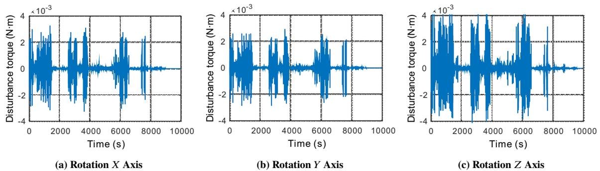
**Fig. 15 Reaction wheel disturbance torques with SMC controller**
