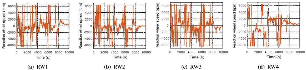
**Fig. 14 Reaction wheel speed histories with SMC controller.**
