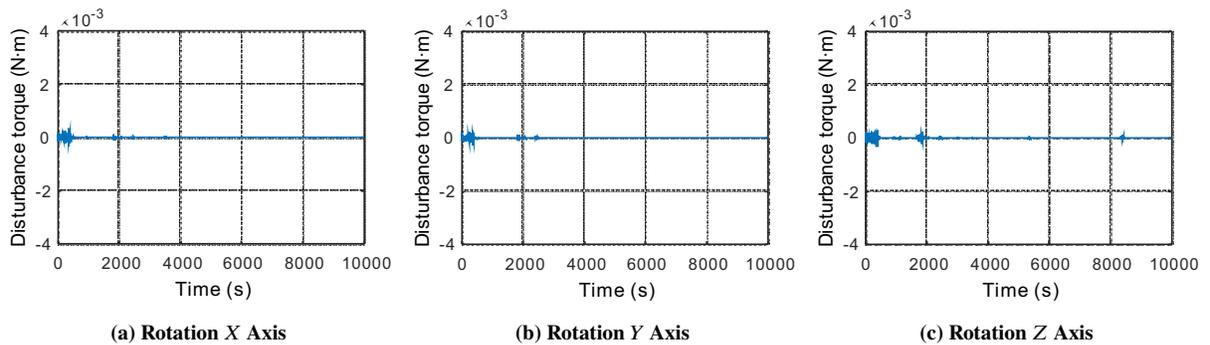
**Fig. 12 Reaction wheel disturbance torques with PD controller and adaptive moment distribution algorithm.**
