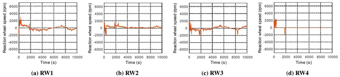
**Fig. 11 Reaction wheel speed histories with PD controller and adaptive moment distribution algorithm.**
