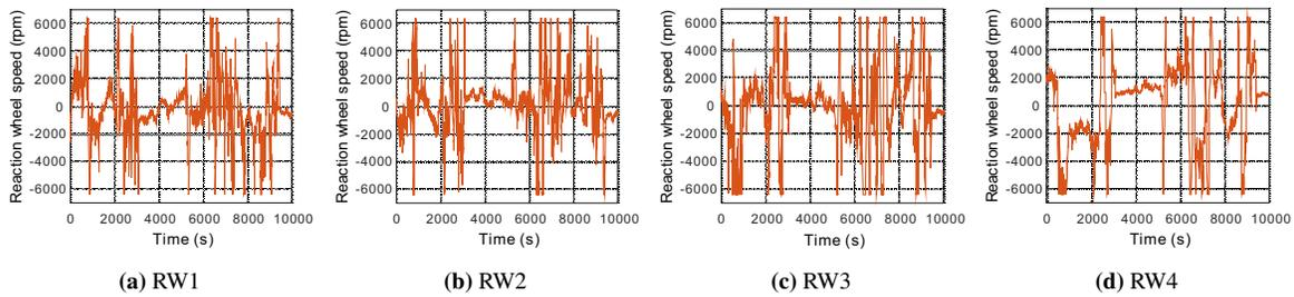
**Fig. 8 Reaction wheel speed histories with PD controller.**
