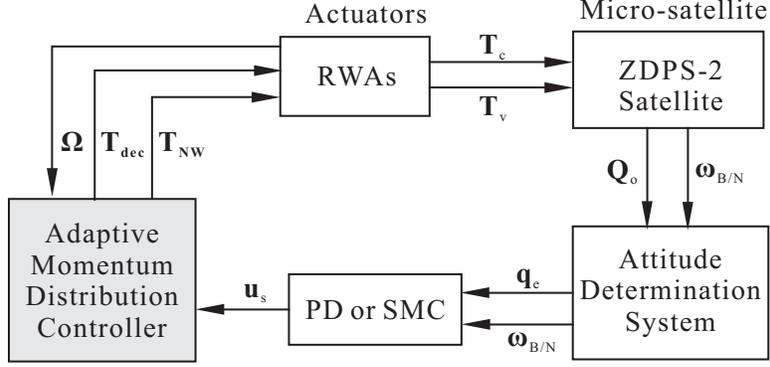
**Fig. 1 Micro-satellite attitude control block diagram.**
