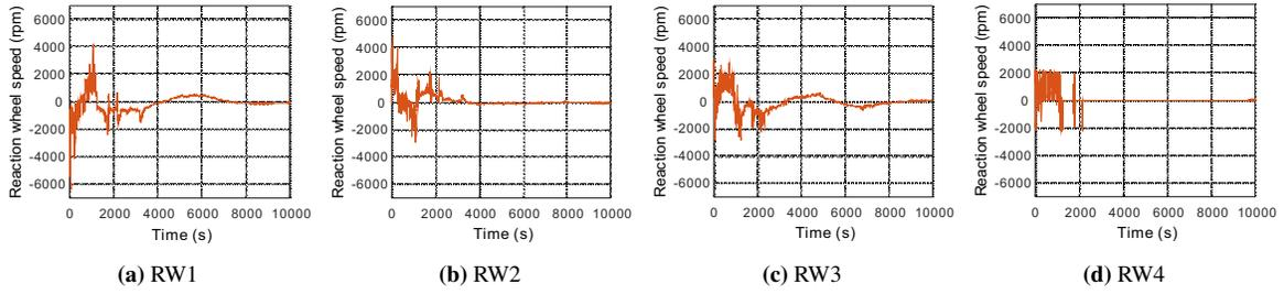
**Fig. 17 Reaction wheel speed histories with SMC controller and adaptive momentum distribution algorithm.**
