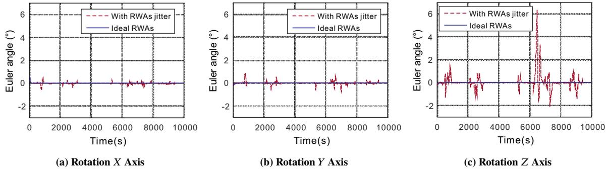
**Fig. 7 The jitter effects on the Euler angles.**
